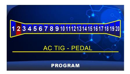
To load a program, scroll to program required and press SAVE/LOAD button
