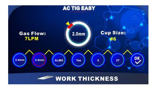
Then use control knob to select work thickness required. 1.0mm, 1.2mm, 1.5mm, 2.0mm, 3.0mm, 4.0mm
