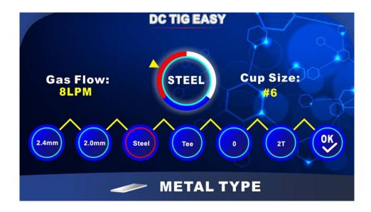
Then use control knob to select metal being welded STEEL = Mild Steel, SS = Stainless Steel
