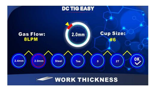
Then use control knob to select work thickness required. 1.0mm, 1.2mm, 1.5mm, 2.0mm, 3.0mm, 4.0mm, 5.0mm, 6.0mm
