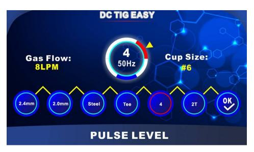
Pulse welding was designed mainly for stainless steel and other exotic materials to control heat input to the metal and decrease heat deformation.
