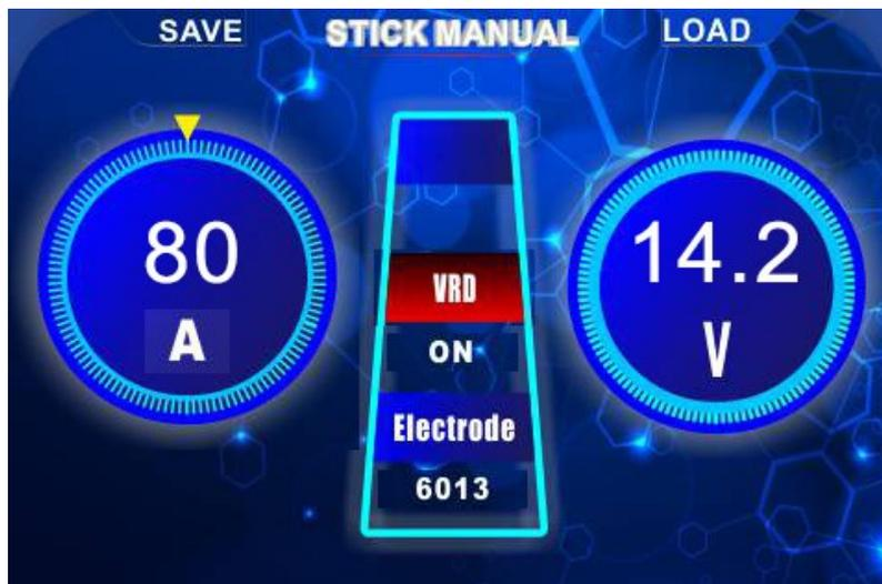
Use the select knob to move between each setting - once setting is highlighted in RED press control knob to highlight setting in RED then turn to change. Once correct setting is selected, press knob again to enter.
