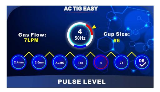
Pulse welding was designed mainly for stainless steel and other exotic materials to control heat input to the metal and decrease heat deformation.
