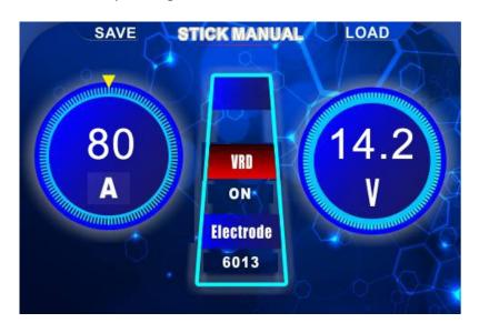
Use the select knob to move between each setting - once setting is highlighted in RED press control knob to highlight setting in RED then turn to change. Once correct setting is selected, press knob again to enter.
