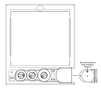
The ADF filter uses two CR2450 lithium cell batteries. Open the battery compartment by sliding the battery tray out. Replace the old battery cells with the new ones. The positive end (+) of the battery must face up. Insert the battery tray back to the cartridge, and then test whether the filter works properly.
