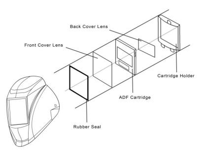
**Replacing the Back Cover Lens:** Take out the filter cartridge. Slide the back safety lens out as shown in the figure below, and then slide a new lens back.
