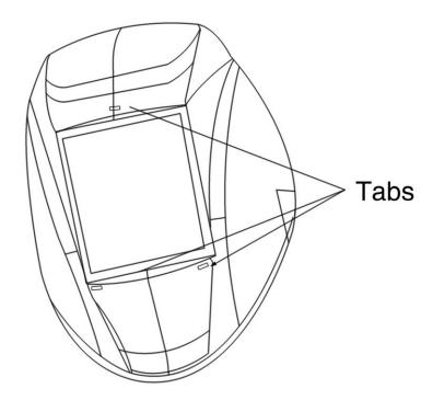
**Removing ADF Cartridge:** Use one finger to press down the tab and at the same time another finger to push off the retainer on the helmet. Start from the bottom and then the top. Remove the cartridge holder and the cartridge.
