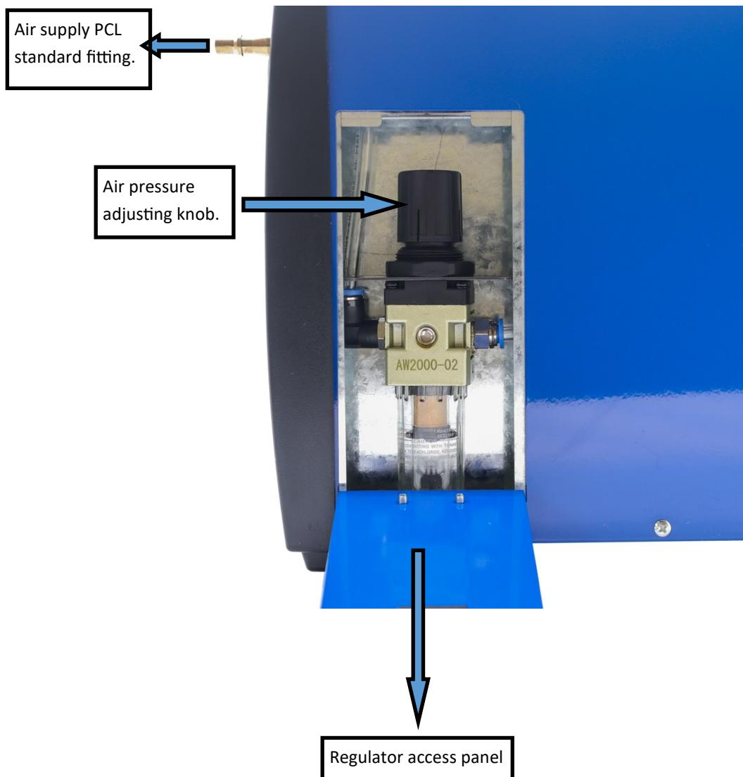
Air pressure adjusting knob - Pull up knob to enable adjustment - once desired air pressure is achieved after pressing trigger quickly so air flows through torch and 70 PSI for cutting is displayed in air pressure LED - now push knob down to lock.
