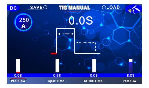
Once you have set the SPOT settings, you return to main TIG screen by turning middle knob to highlight the following icon in RED, then pressing in middle knob. There you can adjust the amperage etc.
