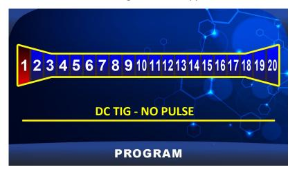
Use the middle control knob to move to required save slot.
