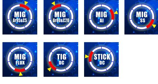
MIG Ar95/C5 - MIG welding with MIG gas - most common. MIG Ar80/C20 - MIG welding with industrial high thickness MIG gas. MIG AL - Aluminium MIG welding with pure argon gas MIG SS - Stainless steel MIG welding MIG Flux - Gasless MIG welding TIG DC - TIG welding with pure argon gas STICK DC - MMA Stick welding
