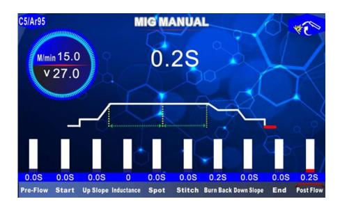
For most common MIG welding we suggest setting all to zero apart from Burnback 0.2s and post flow 0.2s.
