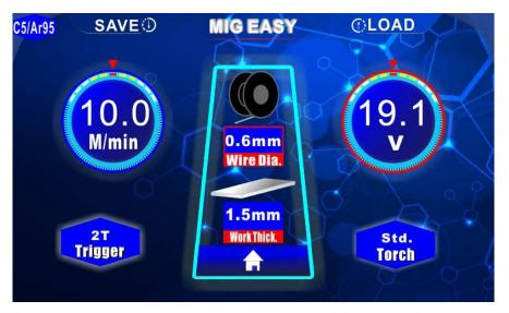
Use the middle knob to cycle through settings, when a setting is highlighted in red, use the left control knob to change setting.
