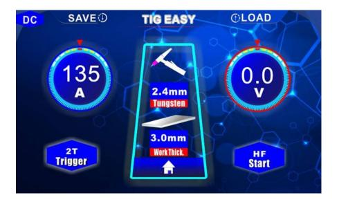
R-Tech Easy mode takes the guesswork out of TIG welding. You normally had to enter desired amperage to weld on manual welders, we have done this for you. You simply select the following from easy to understand screen.
