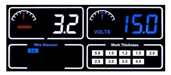
Once you have selected 0.8mm wire size and material thickness the suggested wire speed and voltage will be shown in the display, you are now ready to weld.
