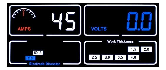
You can trim the welding amperage by using left control knob + /- 10 amps to suit your personal welding travel speed / weld bead.
