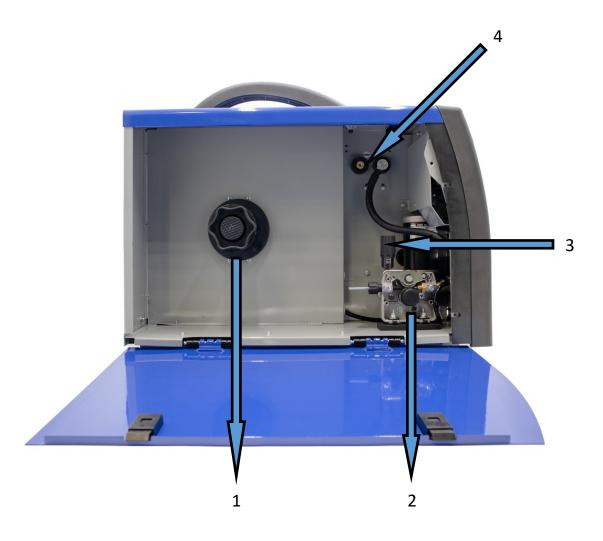
1 - Wire reel retainer. Screw in to retain wire roll adaptor onto wire reel.
