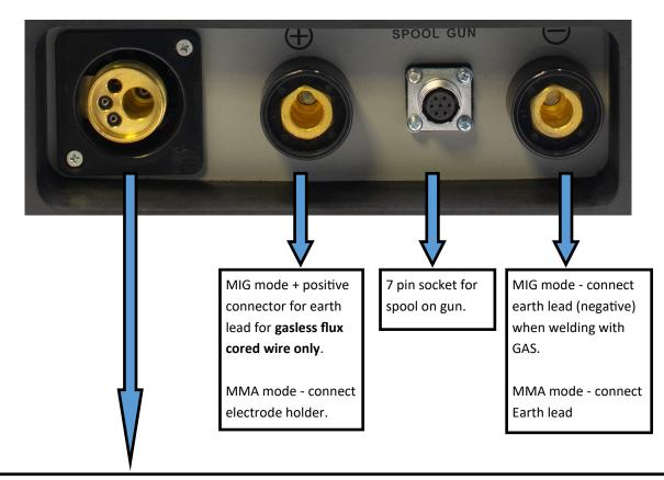
Euro torch connector. Connect Euro type MIG torch to euro torch connector, align torch connector to machine connector and then turn retaining ring clockwise to secure. Ensure torch is secured tightly to avoid weld power problems
