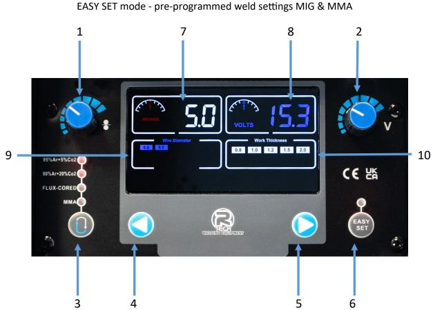
Digital Colour Screen with easy to navigate menu system EASY SET mode - pre-programmed weld settings MIG & MMA
