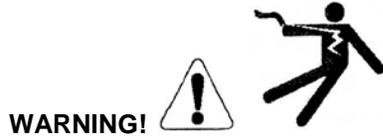
Electric Shock can kill – Only qualified personnel should perform this installation. Turn off input power at the fuse box before working on this equipment. Do not touch electrically live parts. Always connect the machine to an earthed mains supply as per national recommended standards.
