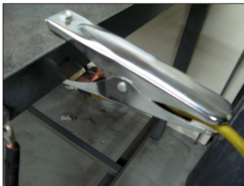
1. Earth clamp secured to the workpiece or bench
