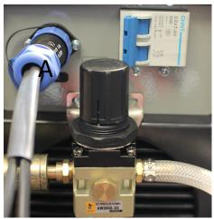
The CNC table, console and PC assembly is now complete, all you need to do now is connect the CNC interface cable A to rear of R-Tech Plasma Cutter, then setup the Plasma Cutter as per the owners manual instructions supplied with P50HF.
