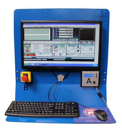
Put PC and CNC control box on rear stand of console.
