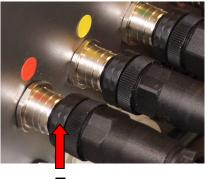
Connect the 4 x motor plugs into sockets which are all colour coded - locate by using alignment lugs on plug and socket, then turn the end ring E on plug to screw it into socket.
