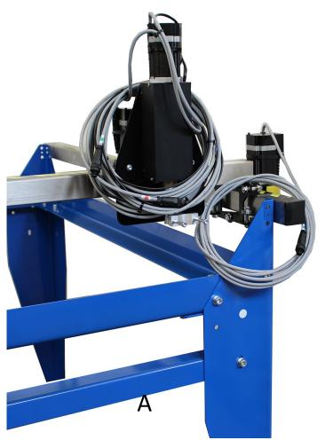
Right side fitted - Shows option water table front beam (A)
