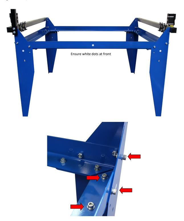
Fit 4 x Allen key bolts, nuts and washer at points show per each corner
