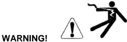
Electric Shock can kill - Only qualified personnel should perform this installation. Turn off input power at the fuse box before working on this equipment. Do not touch electrically live parts. Always connect the machine to an earthed mains supply as per national recommended standards.
