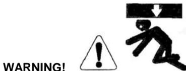
Falling Equipment can cause injury. Never lift welder with gas bottle attached. Never lift above personnel.
