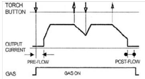
When the trigger mode is in the 4 step position the following sequence will occur
